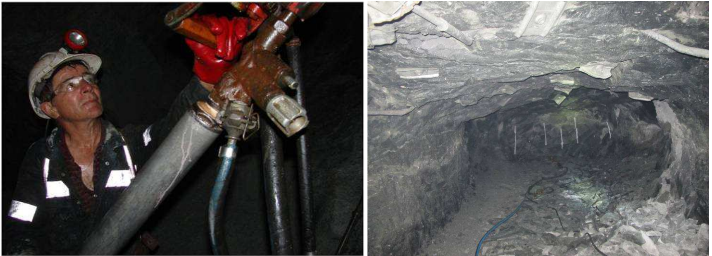
Exhibit 28: An Air-Leg Miner (LHS) and an Air-Leg Mining Face (RHS)
