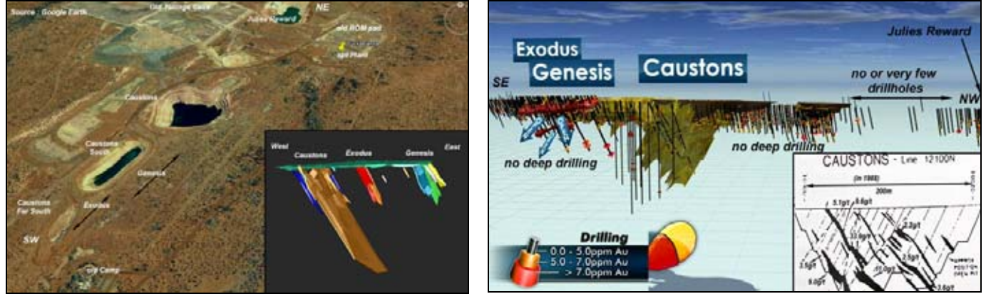
Figure 12. 3d Aerial (Google Earth) View of Caustons, and 3d Schematic & Older (1988) Section of Caustons
